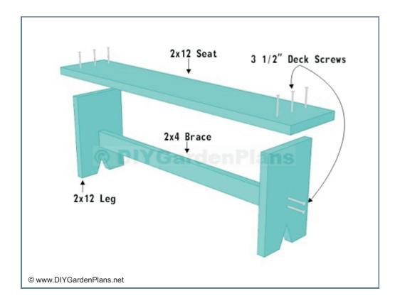
Cut the 8' 2x12 to: One 5' for the seat. Two 1'6" for the legs.
